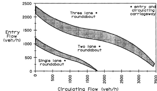
The shaded bands indicate conditions in which either treatment may be suitable depending on the geometry and acceptable operating conditions.
