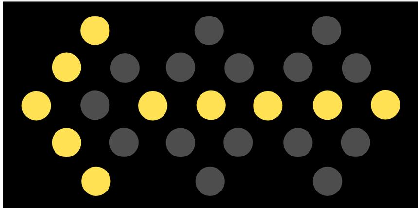
Flashing arrow boards (FABs) are traffic signs with a matrix of lights which can be flashed in unison or in sequential displays. They are very effective both day and night. FAB is possibly a misnomer for this device as it can show both directional arrows and non-directional displays. The FAB term is used for convenience.
