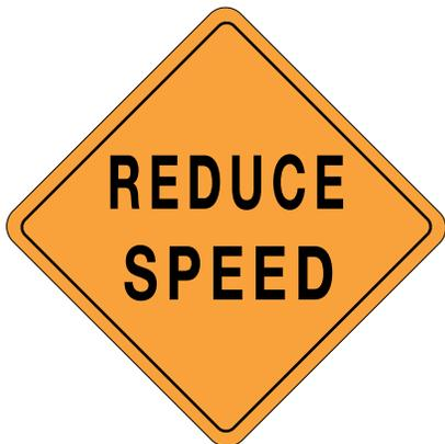
The C-31 sign may be used in conjunction with the C-30 and TW-61L & R signs, in the Advance Warning Area, on multilane highways where the speed limit is 70 km/h or higher. It is not required where a construction speed zone has been established but can be useful in slowing traffic without the imposition of a lower legal speed requirement.
