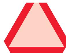
The marker shall also be displayed on the rear of mobile equipment units, involved in road work, which are incapable of moving consistently at speeds above 40 km/h. On such units, the TW-59 marker may be permanently displayed.
