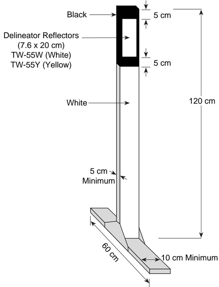
Temporary delineator posts (TDPs) are used to channelize traffic, to separate opposing lanes, to separate lanes of same direction traffic and for outlining work areas. Particularly at night, their use for these purposes may be preferred over Type B or C traffic cones, due to the narrow design and the additional height.
