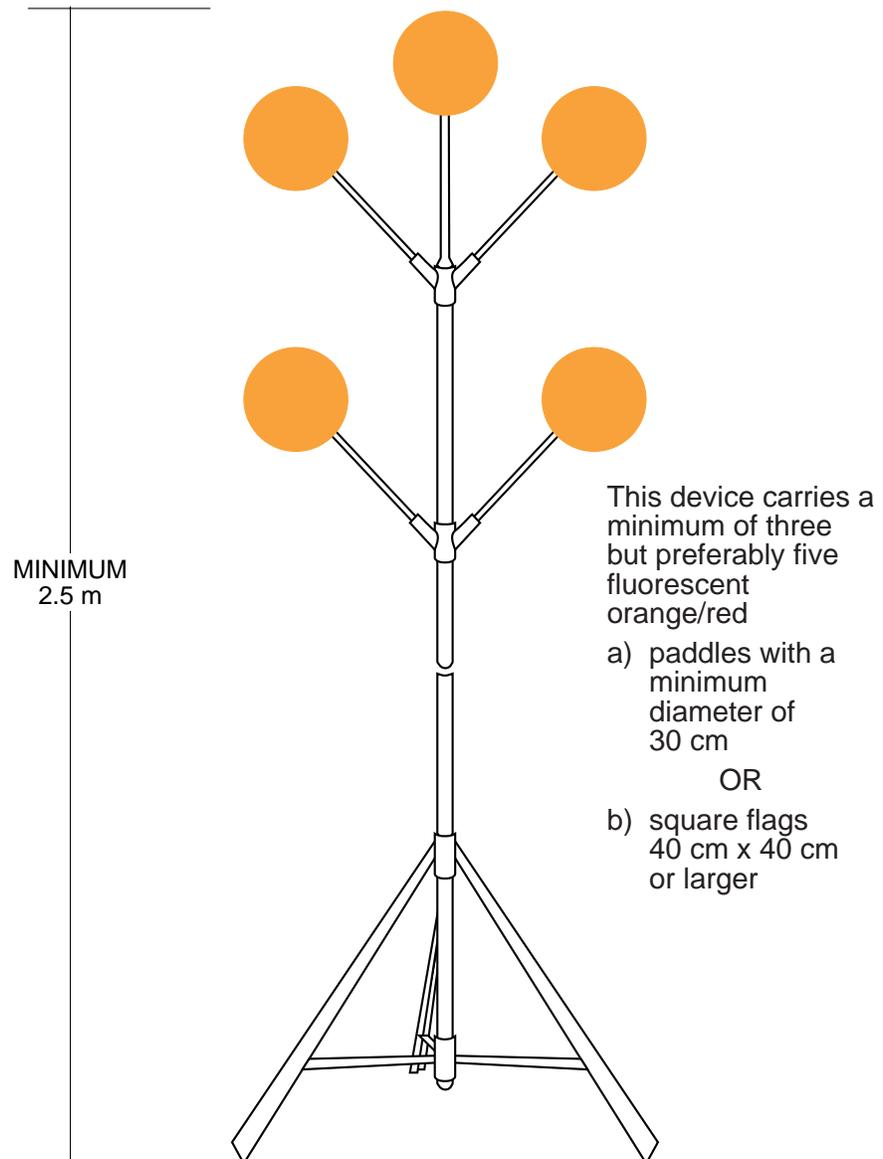
HLWDs are tall portable stands with fluorescent paddles or flags that are visible above traffic and parked cars. They are used only in daylight hours and most often in urban areas; especially where there is insufficient distance to erect all the usual warning signs in advance of work areas. HLWDs may also be used in rural areas to emphasize advance warning signs which could be quite remote from moving work areas and they may be used in work areas where no vehicles are present.
