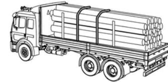
Alternatively, long logs on a frame vehicle may be secured by two or more tiedowns used as wrappers to encircle the entire stack of logs.
