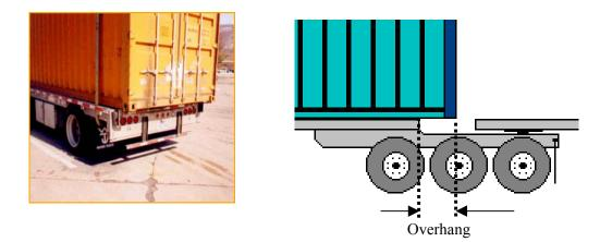
**Comments:** The overhang is measured from the rear of the <u>deck</u> or cargo carrying area of the lead semitrailer on B Trains (not from the extended frame which supports the fifth wheel).
